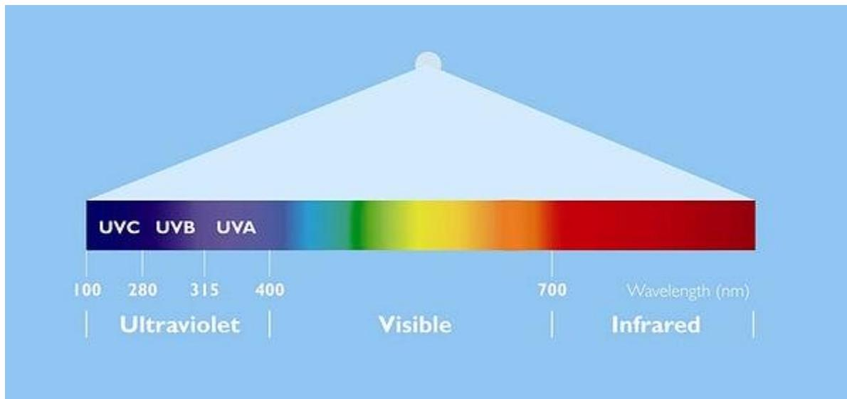
UVGI devices can produce strong enough UVC light in circulating air or water systems to make them inhospitable environments to microorganisms such as bacteria, viruses,
