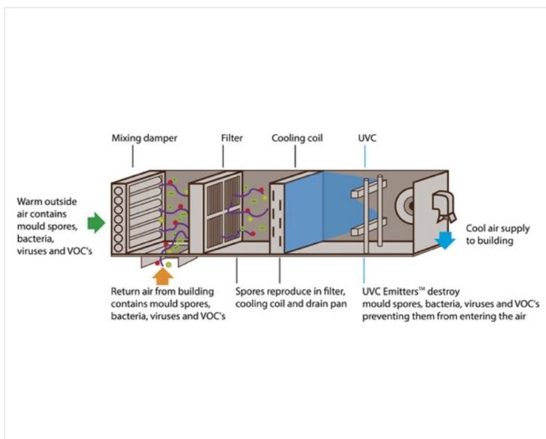
Research has demonstrated up to 99% reductions of molds and bacteria on irradiated surfaces. The effectiveness of UV systems that irradiate microorganisms in flowing air can also be substantial but is less dramatic and depends highly on the microorganism type, air velocity, humidity, the size of the particles carrying the microorganisms, and the UV system design
